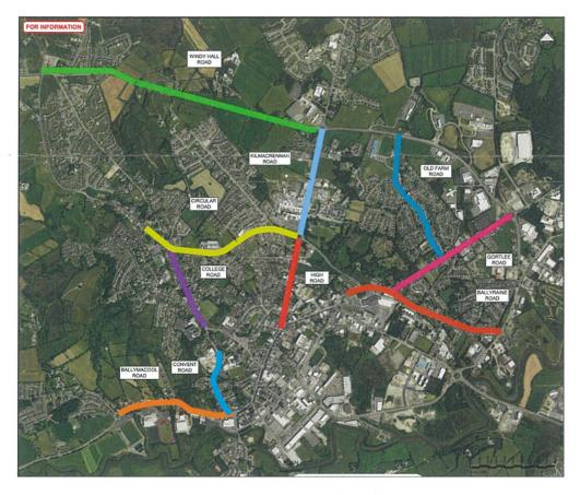
Scheme 04 – L-1006 Convent Road – It is proposed provide a new shared walking and cycling facility on the west side of the carriageway by relocating existing road space to the facility.
